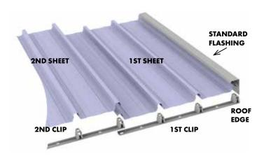
3. Fix the clip as indicated. Ensure the clip is 90° to the edge of the sheet and facing the direction required for laying.
